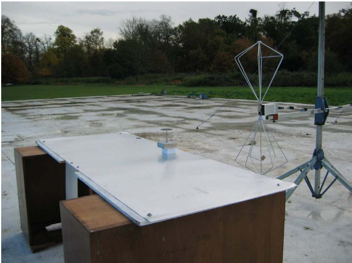
Figure 139 Ground Conducting Bench on an OATS showing the Conducting Straps to Ground
