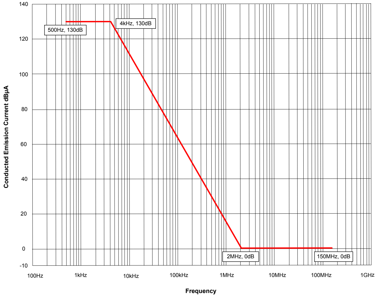
Figure 16 DCE02.A – Class A Limit for Man Worn, Man Portable Land Based Equipment
